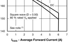
Fig. 4 - Maximum Allowable Case Temperature vs. Average Forward Current
