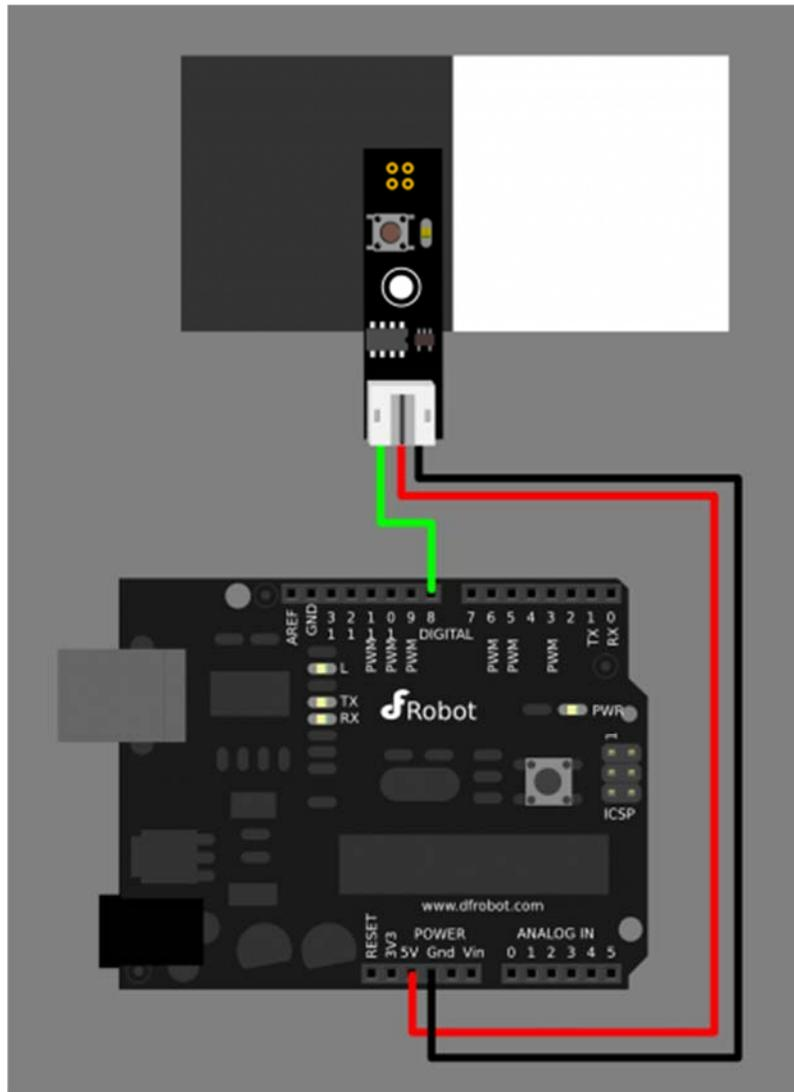
Grayscale Sensor Connection Diagram in digital mode
