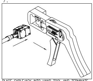
PLACE CABLEJACK INTO HAND TOOL AND TERMINATE.
