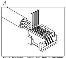
TRIM BOTTOM ROW OF CONDUCTORS FLUSH WITH LOADBAR.
