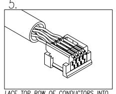
LACE TOP ROW OF CONDUCTORS INTO LOADBAR. TRIM TOP ROW OF CONDUCTORS FLUSH.
