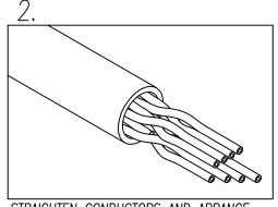
STRAIGHTEN CONDUCTORS AND ARRANGE ACCORDING TO APPROPRIATE WIRING DIAGRAM ON THE BACK OF THIS SHEET. TRIM OFF BOTTOM ROW OF CONDUCTORS AT A SLIGHT ANGLE TO FACILITATE EASIER LOADING.
