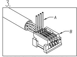
BEND TOP ROW OF CONDUCTORS BACK 90 DEGREES (A). LOAD BOTTOM ROW OF CONDUCTORS INTO LOADBAR (B).
