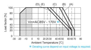
Fig.4.5 Derating curve depend on ambient temperature
