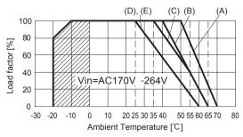
Fig.4.8 Derating curve depend on ambient temperature
