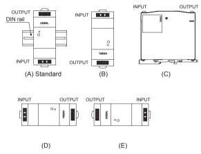
Fig.4.1 Mounting orientation
