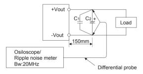
C1:Film capacitor 0.1 µ F C2:Aluminum electrolytic capacitor 22 µF
