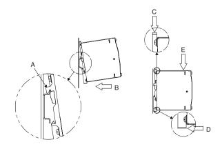
Fig.4.2 Installation method
