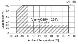
Fig.4.10 Derating curve depend on ambient temperature
