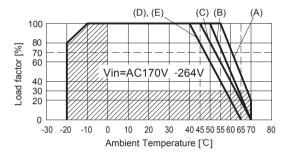
Fig.4.6 Derating curve depend on ambient temperature
