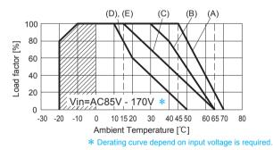
Fig.4.7 Derating curve depend on ambient temperature
