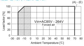
Fig.4.11 Derating curve depend on ambient temperature
