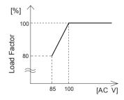
Fig.4.4 Derating curve depend on input voltage
