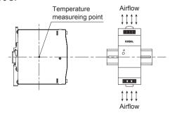
Fig.4.12 Temperature measurement point (Forced air)
