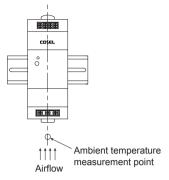
Fig.4.9 Ambient temperature measurement point
