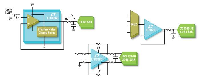
Linear Technology offers a wide range of amplifiers for driving the industry's highest performance successive approximation register (SAR) ADCs, including:
