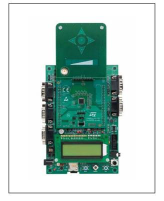
The kit contains an STM8/128-EVAL board, and an STM8S touch sensing evaluation daughterboard (STM8Sxxx-TS1) which provides an evaluation platform for the resistor-capacitor acquisition principle.
