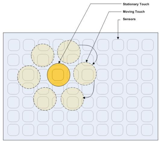
Crosstalk refers to the sudden rise/decrease in the position jitter of the stationary touch when the other touch comes closer to the stationary touch. Cross-talk can be measured/expressed in the same method as Jitter. Shadowing problem refers to the disappearance of a stationary touch when the other touch scrolls nearer to the stationary touch. Both the factors can be tested and monitored by rotating one touch 360 degrees against the stationary touch.
