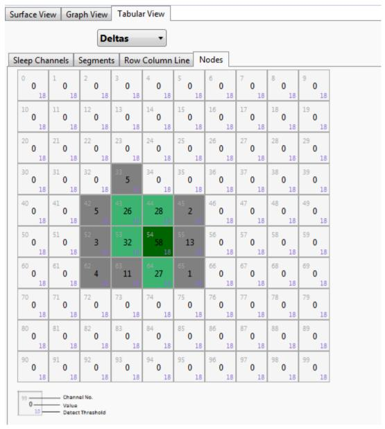
The sensor node which has the highest peak delta will be shown in dark green colour. The sensor nodes whose delta is above the detect threshold are highlighted with light green color. And the nodes which has the delta below Detect threshold are highlighted with light grey colour.
