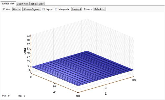
In the surface view, X-axis, Z-axis shows row sensor nodes and column sensor nodes of surface respectively. Y-axis represent delta value of the touched sensor nodes.
