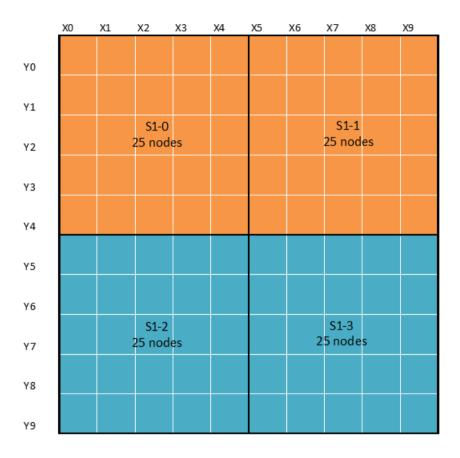
The Lumped Sensors arrangement for segment sensors is formed by splitting the Sleep Sensors along the other grouping axis. For example: If Sleep sensor grouping is along the Y axis, then the Lumped Sensors will be split along the X axis to form Segment Sensors.
