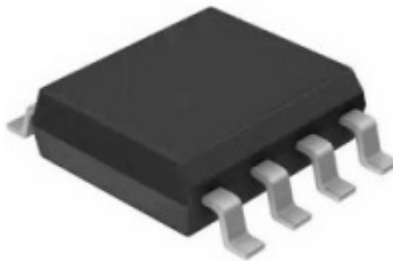
Typical IC package accepted (SOIC-8)
