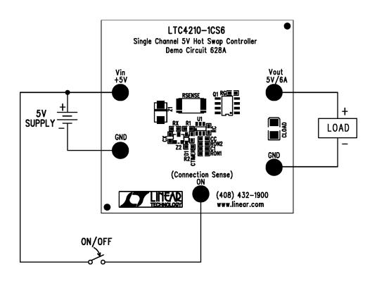
Figure 1. Proper Measurement Equipment Setup
