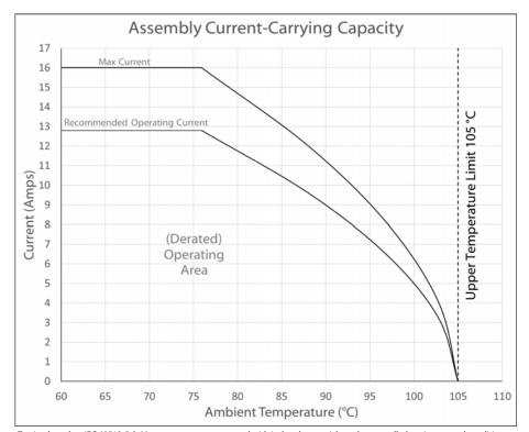
Testing based on IEC 60512-5-2. Max current curve generated with isolated test article under controlled environmental conditions, and does not take into account external factors such as housings or circuitry. Recommended operating current curve (derated to 80% of max values) accounts for external factors, manufacturing variation, and error in temperature measurements.
