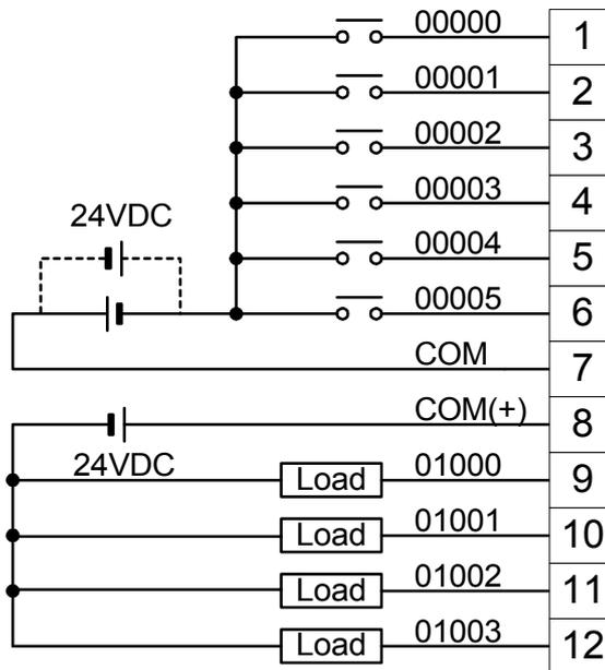
Do not exceed the output capacity or the maximum common current for transistor outputs shown in the following table.
