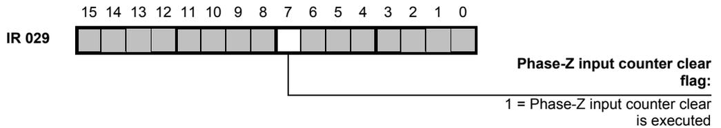
**Note** The flag is reset when the Phase-Z input counter clear function is enabled again.
