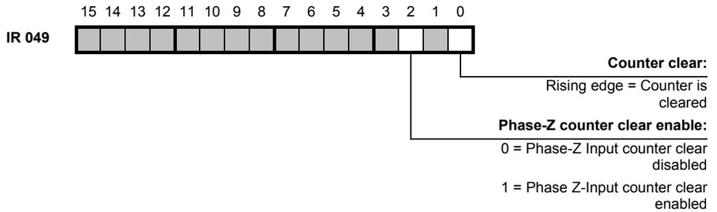
**Caution** While the Phase-Z counter clear function is enabled, changes to the other bits in IR 049 are prohibited.
