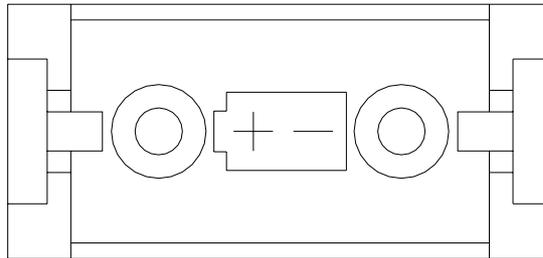
3. Install the new battery. Be sure the battery is positioned in the correct way, according to the picture in the holder.
