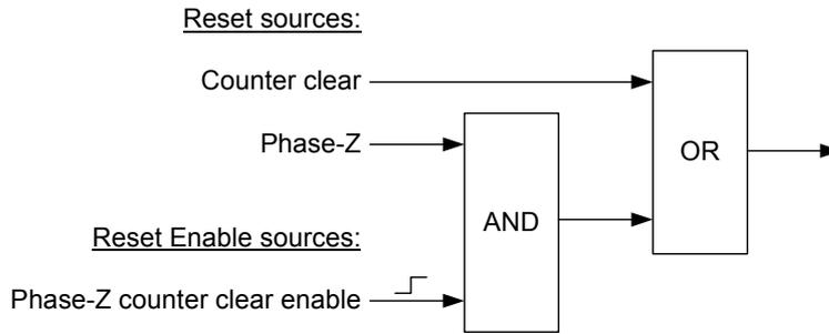
**Note** When the counter has been cleared with the Phase-Z input, the function is disabled. To enable the function again the enable bit must be cleared and set again.
