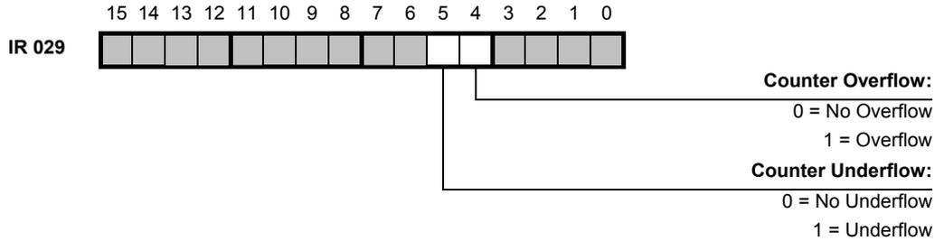
The Counter can be cleared by using the Counter clear bit. The Over- and Underflow flags can be cleared by using the Over- and Underflow reset bits. The Counter can be enable and disabled with the Counter Disable bit.
