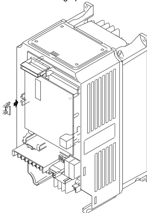
6. Attach the FE-cable of the PLC option board to the FE-connection screw on the terminal-board:
