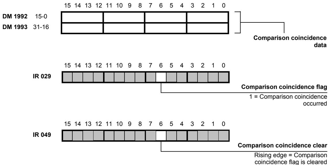
**Caution** The Comparison coincidence clear function is executed when a rising edge is generated (0 → 1). Keep this bit high during 1 PLC cycle only. It is prohibited to use the Comparison coincidence clear function while the Phase-Z counter clear function is enabled (IR 049.02).
