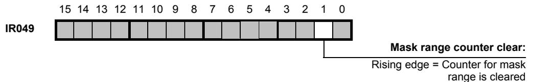
**Caution** The Mask range counter clear function is executed when a rising edge is generated (0 → 1). Keep this bit high during 1 PLC cycle only. It is prohibited to use the Mask rang counter clear function while the Phase-Z counter clear function is enabled (IR 049.02).
