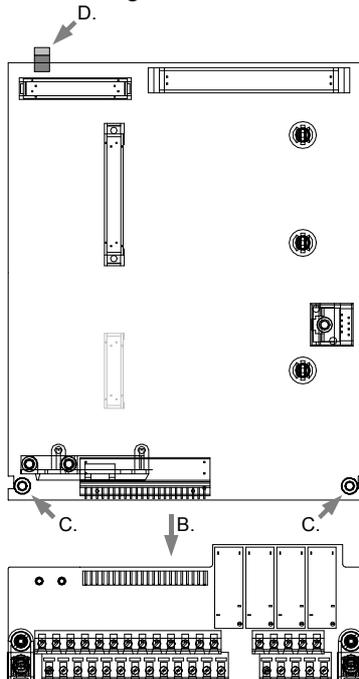
**B.** Release the screws of the controller-board.
