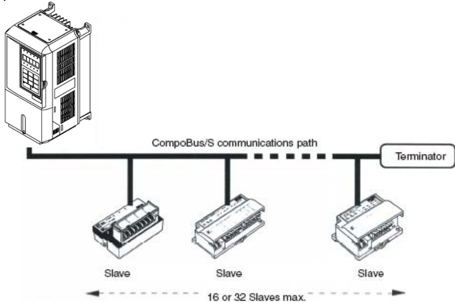
Use a Programming Device to set the maximum number of Slaves in DM 6603 of the PLC Setup, as shown in the following table.
