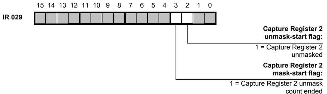
**Note** The Unmask- and Mask-start flags are active during 1 PLC cycle only.
