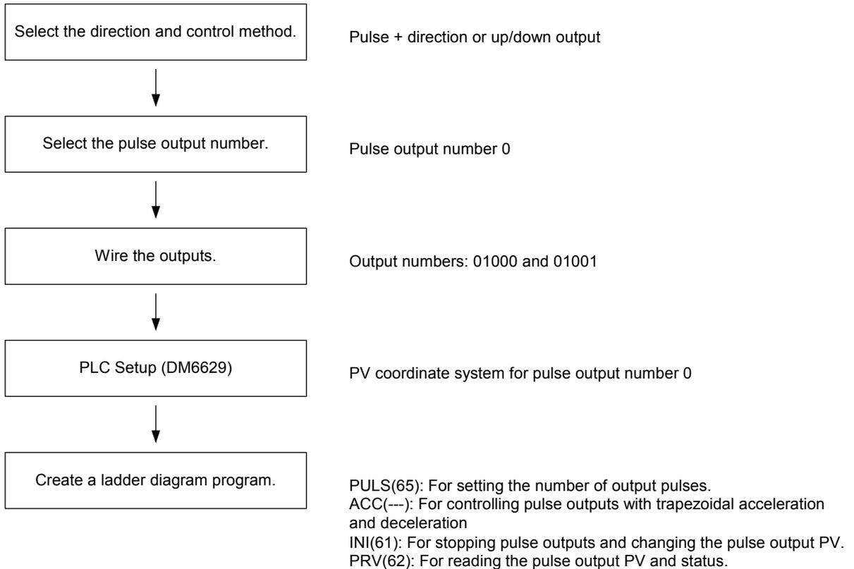
Pulse Outputs With Trapezoidal Acceleration and Deceleration
