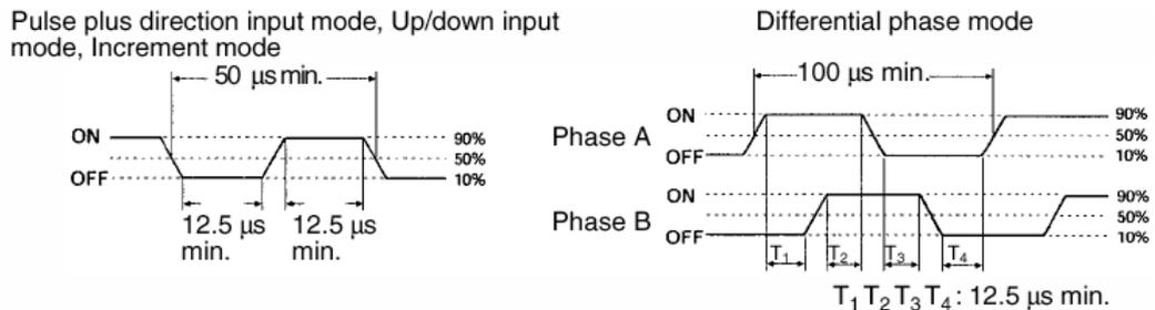
The minimum pulse width for input 00002 (Z-phase input) is as follows:
