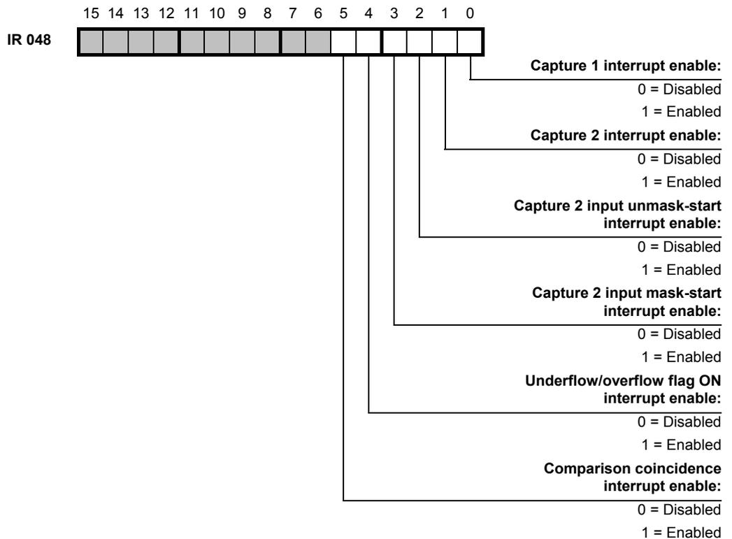
**Note** When more than one event can generate an interrupt, the exact event cannot be determined in the interrupt program: the status of the corresponding flags are not updated yet.
