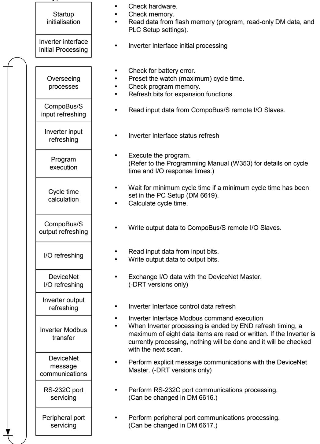
The cycle time can be read from a Programming Device. AR 14 contains the maximum cycle time and AR15 contains the present cycle time in multiples of 0.1 ms.
