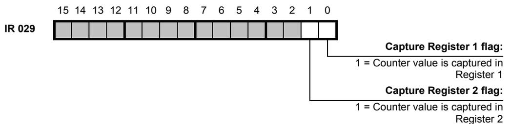
**Note** The Capture Register flags are cleared automatically: the flags are active during one scan only.
