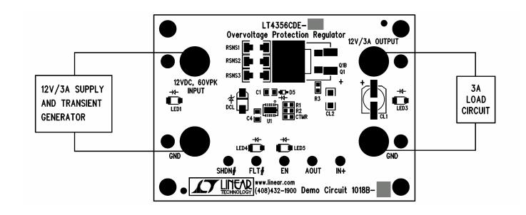
Figure 1: Proper Measurement Equipment Setup
