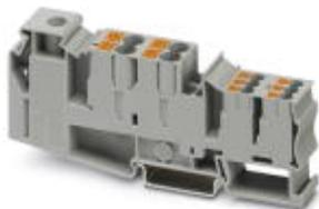
Potential collective terminal, nom. voltage: 1000 V, nominal current: 105 A, connection method: Screw connection, Push-in connection, number of connections: 11, cross section: 1.5 mm<sup>2</sup> - 50 mm<sup>2</sup>, AWG: 16 - 1/0, width: 16.3 mm, color: gray, mounting type: NS 35/7,5, NS 35/15
