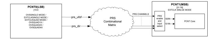
Figure 16.14. PCNT Cascading to two 16-bit PCNT to form a 32-bit PCNT
