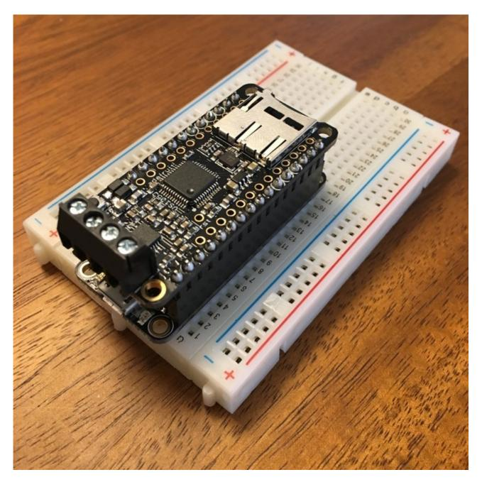
Now, grab a small screwdriver and attach the speaker wires to the MusicMaker FeatherWing terminals. We are only going to use the one speaker, so it really doesn't matter which speaker channel you choose. You can put it in the right, or left side. Just make sure to connect the red (positive) wire to one of the outside terminals, and the black (negative) wire to one of the inside terminals.
