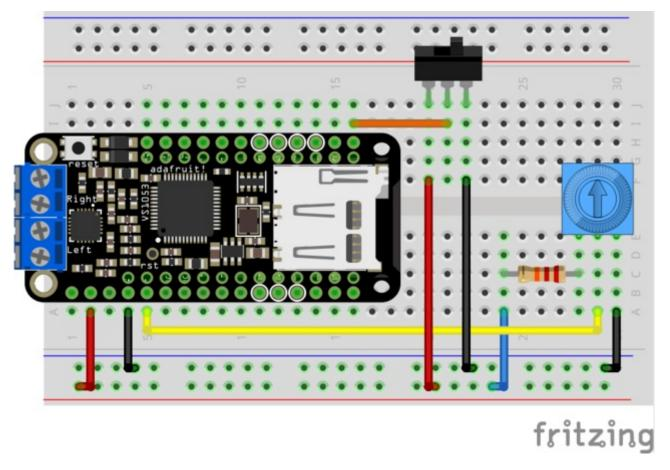
Power up your radio and flip the switch to the power side to turn it on. Try flipping the switch once the radio starts playing to see if it shuts off.
