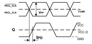
Figure 5. LVCMOS Propagation Delay (TPD) Test Reference
