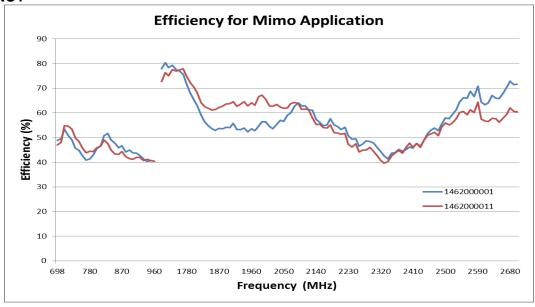
FIGURE 7.2 EFFICIENCY OF 1462000001 AND 1462000011 ANTENNAS
