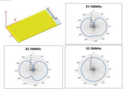
FIGURE 6.1 RADIATION PATTERN OF ATNENNA AT 700MHZ IN FREE SPACE
