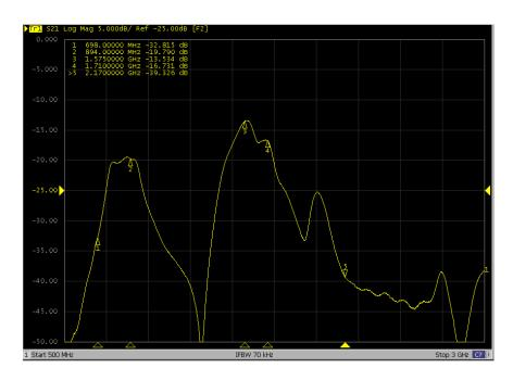
FIGURE 7.4 ISOLATION OF 1462000001 AND 1462000011 ANTENNAS
