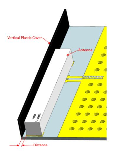
FIGURE 4.3 DIFFERENT DISTANCE BETWEEN VERTICAL PLASTIC COVER AND ANTENNA
