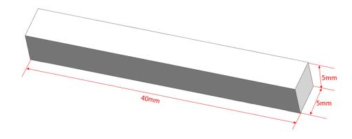
FIGURE 8.2 OVERALL ANTENNA SIZE (1462000001 and 1462000011)
