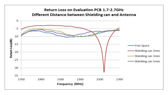
FIGURE 4.1.2 RETURN LOSS COMPARISON AT 1.7-2.7GHz BAND OF DIFFERENT SHIELDING CAN DISTANCE FROM ANTENNA
