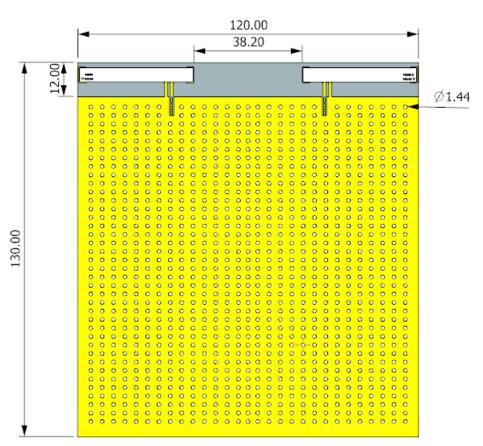
FIGURE 2.2 RECOMMENDED PCB LAYOUT FOR MIMO APPLICATION
