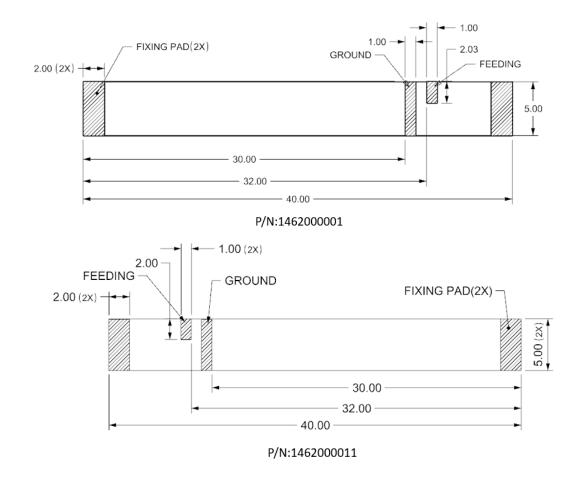
FIGURE 8.4 PADS OF PRODUCT FOR SOLDERING
