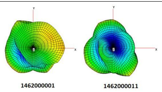
FIGURE 7.6.6 3D RADIATION PATTERN AT 1990MHZ OF 1462000001 AND 1462000011 ANTENNAS
