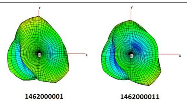
FIGURE 7.6.4 3D RADIATION PATTERN AT 1710MHZ OF 1462000001 AND 1462000011 ANTENNAS
