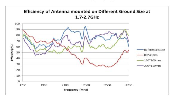
FIGURE 4.5.4 EFFICIENCY COMPARISON AT 1.7-2.7GHZ OF ANTENNA MOUNTED ON DIFFERENT SIZE GROUND
