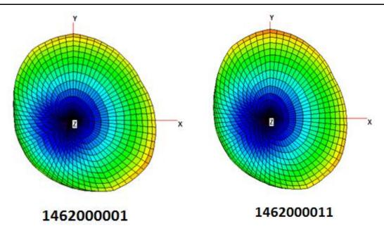
FIGURE 7.6.2 3D RADIATION PATTERN AT 820MHZ OF 1462000001 AND 1462000011 ANTENNAS
