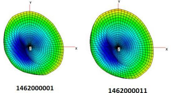
FIGURE 7.6.3 3D RADIATION PATTERN AT 960MHZ OF 1462000001 AND 1462000011 ANTENNAS
