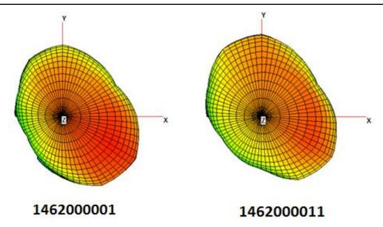
FIGURE 7.6.8 3D RADIATION PATTERN AT 2500MHZ OF 1462000001 AND 1462000011 ANTENNAS
