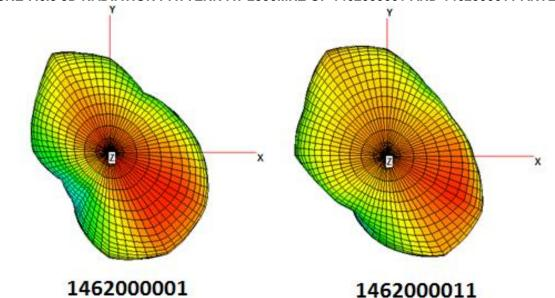
FIGURE 7.6.9 3D RADIATION PATTERN AT 2700MHZ OF 1462000001 AND 1462000011 ANTENNAS
