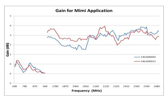
FIGURE 7.3 PEAK GAIN OF 1462000001 AND 1462000011 ANTENNAS
