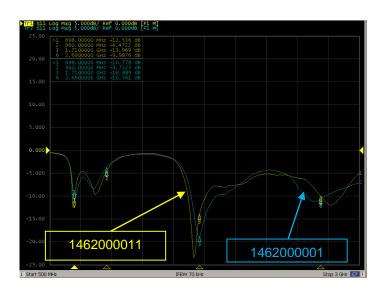
FIGURE 7.1 RETURN LOSS OF 1462000001 AND 1462000011 ANTENNAS
