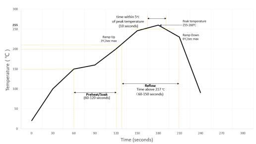
FIGURE 8.1 RECOMMENDED SMT REFLOW PROFILE
