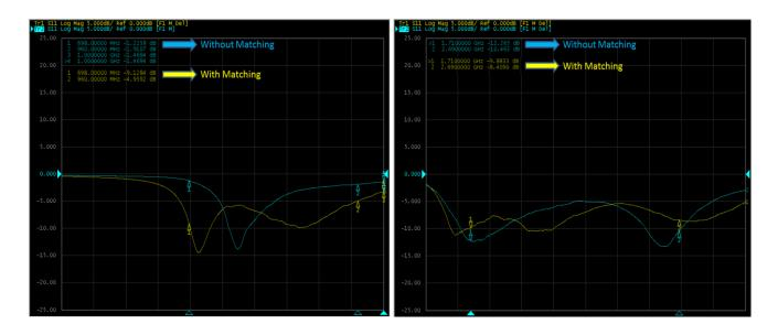
FIGURE 5.7 RETURN LOSS OF ANTENNA WITH AND WITHOUT MATCHING ON 130\*60MM GROUND
