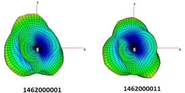
FIGURE 7.6.5 3D RADIATION PATTERN AT 1850MHZ OF 1462000001 AND 1462000011 ANTENNAS
