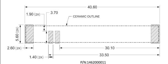
FIGURE 8.5 RECOMMENDED FOOTPRINT ON PCB FOR SOLDERING
