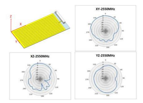
FIGURE 6.5 RADIATION PATTERN OF ATNENNA AT 2550MHZ IN FREE SPACE
