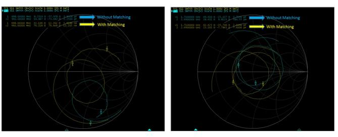
FIGURE 5.8 SMITH CHART OF ANTENNA WITH AND WITHOUT MATCHING ON 130\*60MM GROUND
