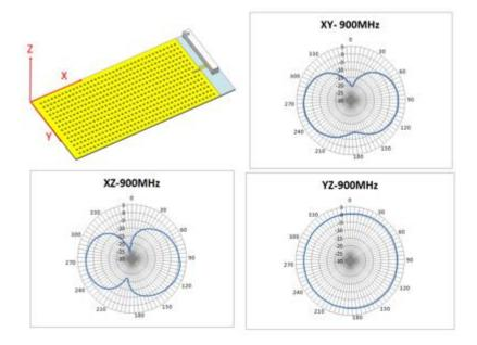
FIGURE 6.2 RADIATION PATTERN OF ATNENNA AT 900MHZ IN FREE SPACE
