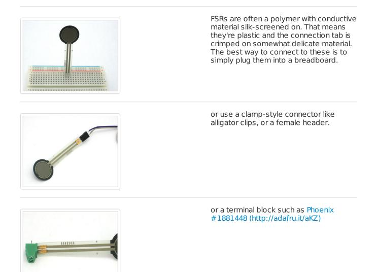
It is possible to solder onto the tabs but *you must be very fast* because if your iron is not good quality or you dally even a few seconds, you will melt the plastic and ruin the FSR! **Don't attempt to solder directly to your FSR unless you are absolutely sure you have the skills to do so.**
