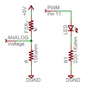
This sketch will take the analog voltage reading and use that to determine how bright the red LED is. The harder you press on the FSR, the brighter the LED will be! Remember that the LED has to be connected to a PWM pin for this to work, I use pin 11 in this example.
