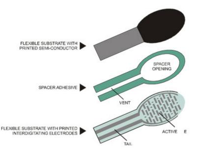
FSRs are basically a resistor that changes its resistive value (in ohms  $\Omega$ ) depending on how much it is pressed. These sensors are fairly low cost, and easy to use but they're rarely accurate. They also vary some from sensor to sensor perhaps 10%. So basically when you use FSRs you should only expect to get *ranges* of response. While FSRs can detect weight, they're a bad choice for detecting exactly how many pounds of weight are on them.
