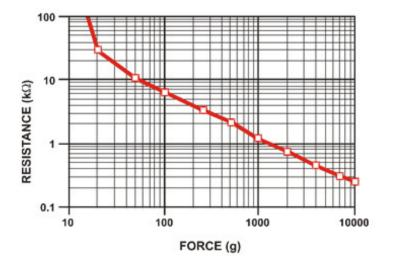
It is important to notice that the graph isn't really *linear* (its a log/log graph) and that at especially low force measurements it quickly goes from infinite to  $100K\Omega$ .
